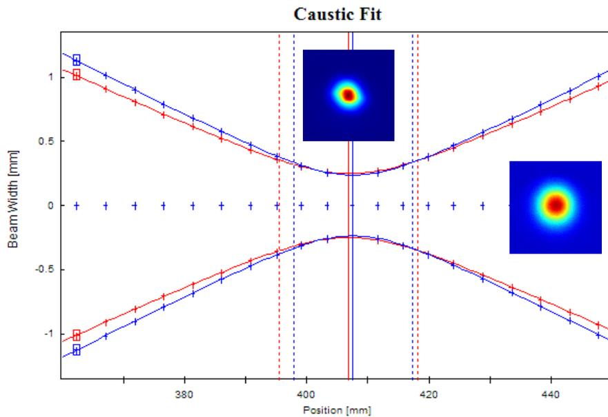
Figure 3. Caustic plot for single laser cavity showing beam profiles in near and far field at 10 kHz.
