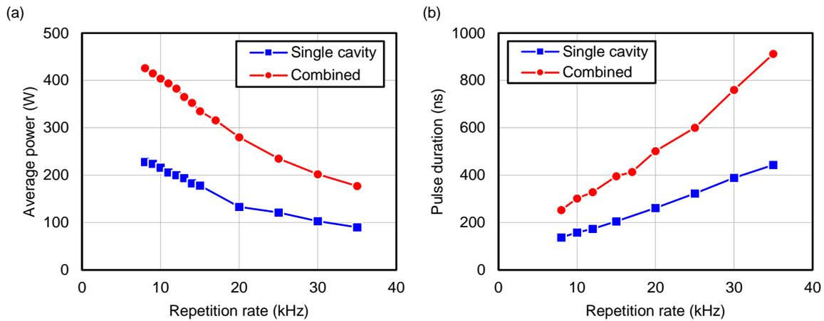
Figure 6. Average power (a) and pulse duration (b) vs pulse repetition rate for single and combined cavities with the delay set to equal one single cavity pulse duration.
