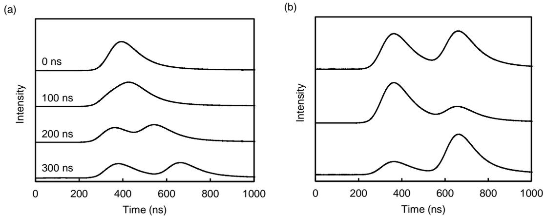
Figure 7. Shape of combined pulse for different delays (a) and shape of combined pulse with 300 ns delay and changing the attenuator values for the two lasers (b).
