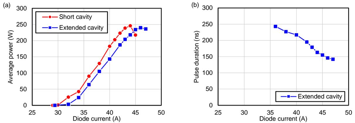
Figure 4. Single cavity power curve for single and extended cavity (a) and pulse duration vs diode current or extended cavity (b) at 10 kHz.
