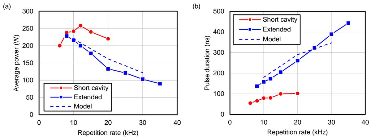
Figure 5. Single cavity average power (a) and pulse duration (b) as a function of pump current for short and extended cavity at 10 kHz, compared with GLAD model for extended cavity
