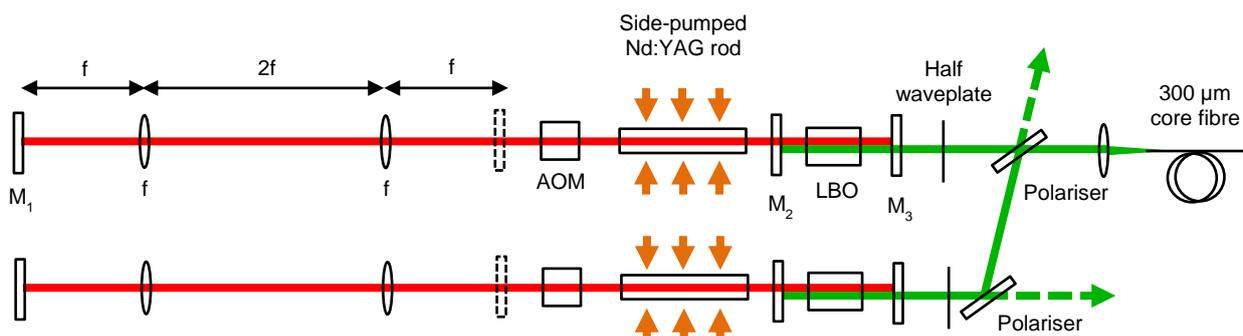
Figure 2. Layout of intracavity frequency-doubled laser showing optimised position of high reflector as dashed line and extended position as solid line.
