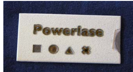
Figure 2 Thermal Barrier Coat (TBC) Milling
