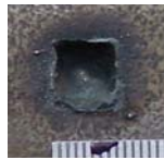
Figure 1c I = 1.2 \times 10^7 \text{W}/\text{cm}^2 \text{MRR} = 49.4 \text{mm}^3/\text{min}
