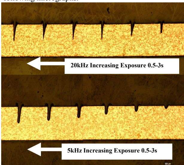
Fig. 7: Kerf Geometry with Exposure for AO1G (low M^2 )
