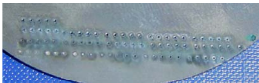
Figure 11: Pierce-through test matrix with air assist gas.
